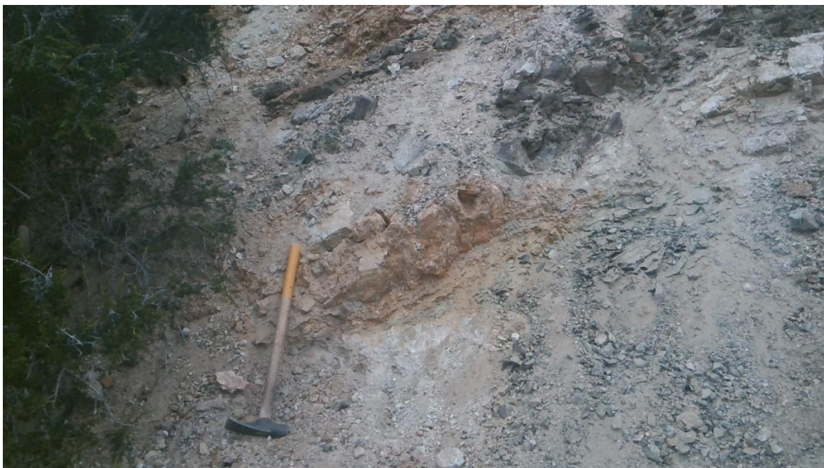
Mineralized veins in pit wall: chip sample here returned 0.40 m @ 46.3 g/t Au
