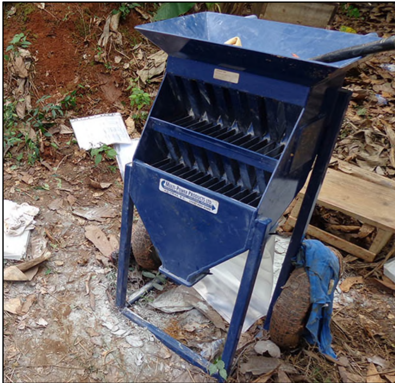
Figure 41: A Jones 3-tier Riffle Splitter
