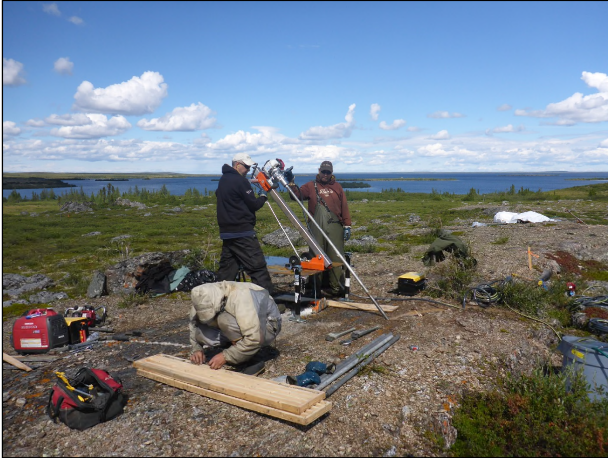
Figure 13: Packsack diamond drill, Metro Drilling, 2017 drill program
