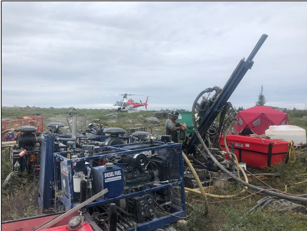
Figure 15: Midnight Sun Drilling: "Hornet " reverse-circulation rotary percussive drill (photo by Jordan Crook)
